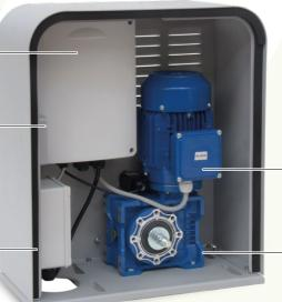
Gearmotor with integrated ventilation, available in 230V 3  $\sim$  and 380 VAC versions
